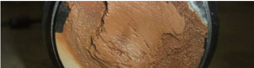
Debris Buildup Around the Detection Section
