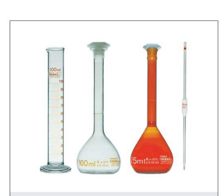
Volumetric Glassware (Class A) Certified volumetric cylinders, volumetric flasks, & pipettes etc.
