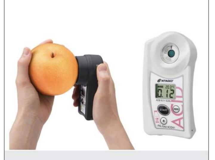
**Portable Meters** For acidity measurement, non destructive brix in fruit etc.
