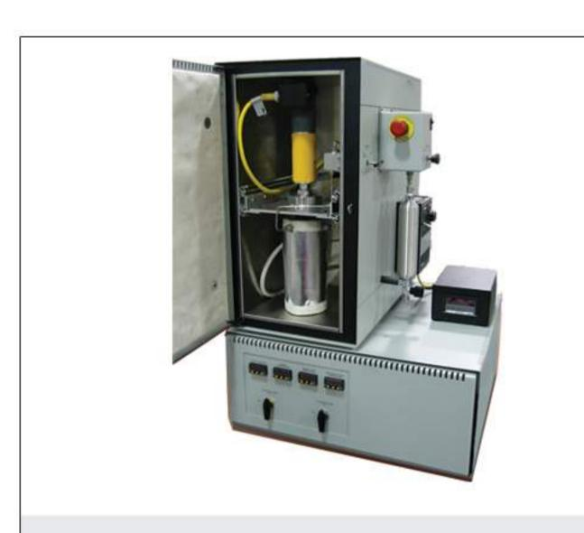
Supercritical Fluid Extractors
